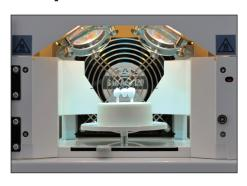
Four powerful halogen lamps, 150 W each with a light wave spectrum of 400-550 nanometres, guarantee efficient curing in the compact polymerisation chamber.
