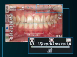
Choose the magnification ratio / range by rotating dial key, icons above pre-set magnification ranges help determine and select range easily.
