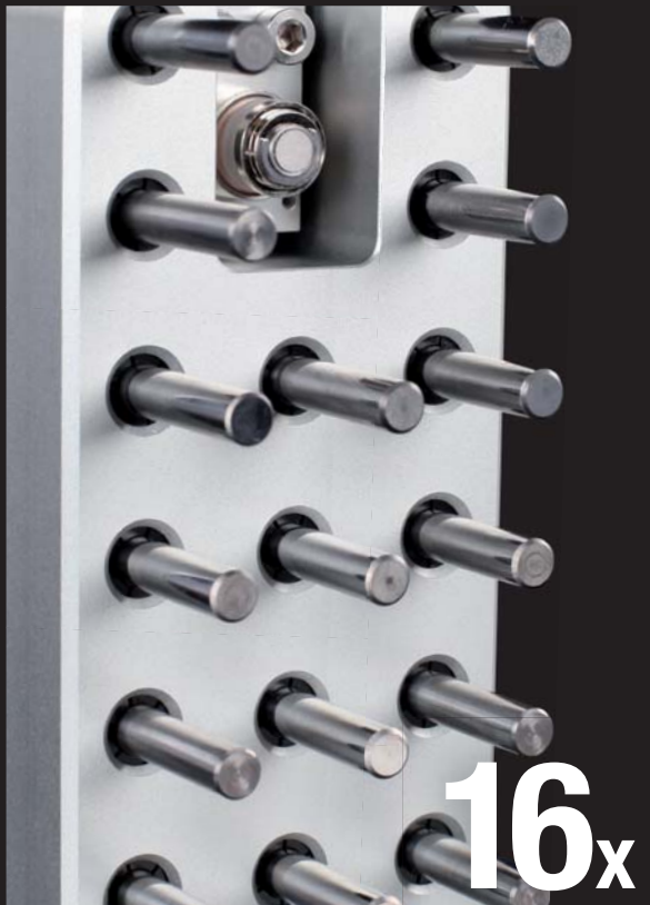
Tool changer on Milling Unit M5 - UPGRADABLE
